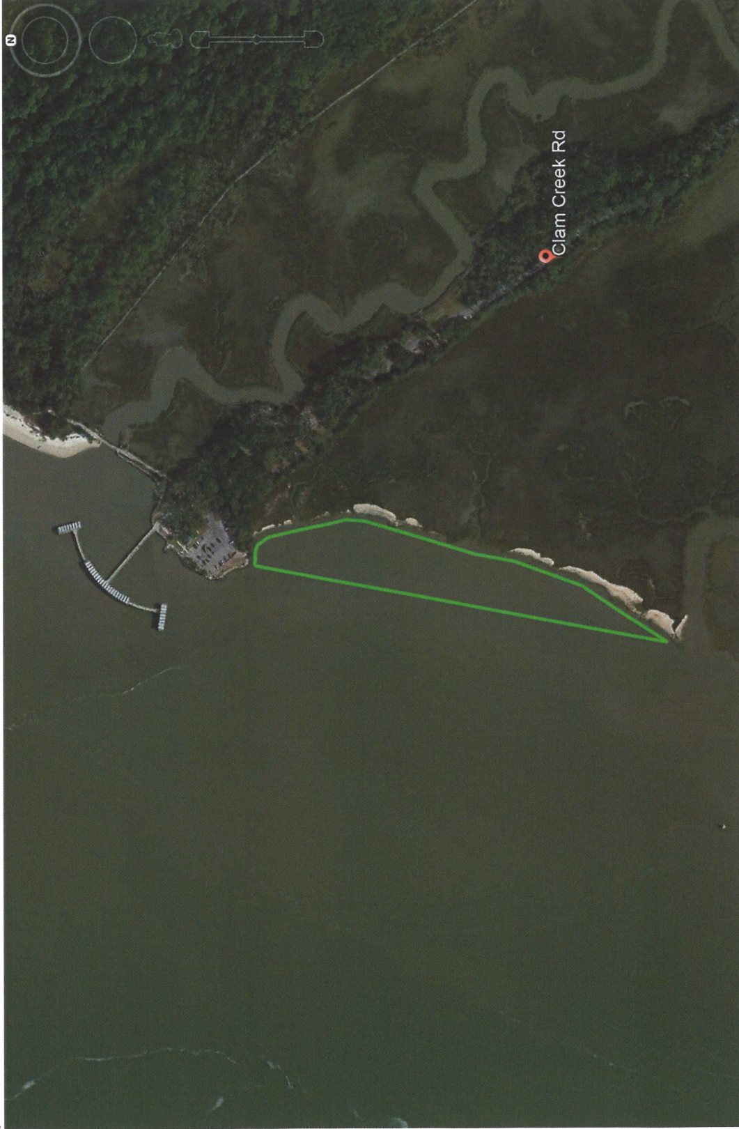
Figure 3. Current site conditions and proposed maximum extent (green outline) of beneficial use placement. Priority for shoreline protection is highest at the north end of this area.
